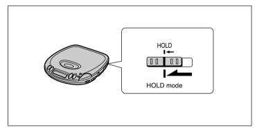
This function causes the unit to ignore short, accidental button presses. (The disc lid can still be opened and closed.)
